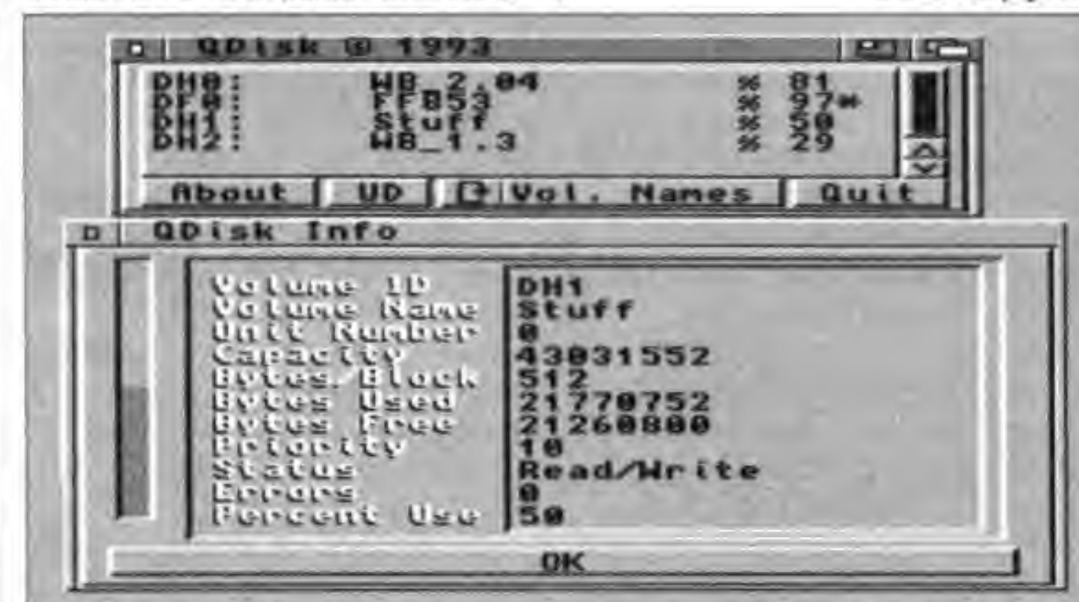
QDisk gives you a clear and useful display of detailed information on any volumes – hard disks, floppies and so on – that are attached to your system.
